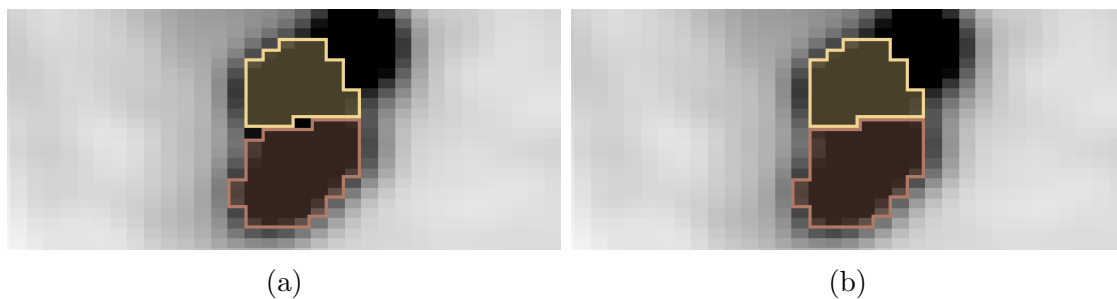
Figure 2.19: A case where a segmentation of two adjacent objects leaves a gap between them. l_{new} is the red label. (a) The single-voxel gaps are visible. (b) The gaps are filled after the sealing is complete.
